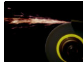
Fig (17) : Why do metal splints rush straight at tangential velocities when using the electric sharpener?
